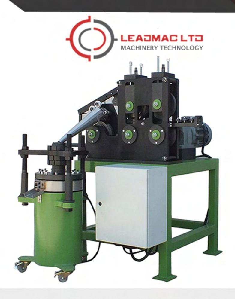
Leadmac's buck shot machine has been designed accurately to produce of buck shots by pressing lead wire with cold shaping system.
